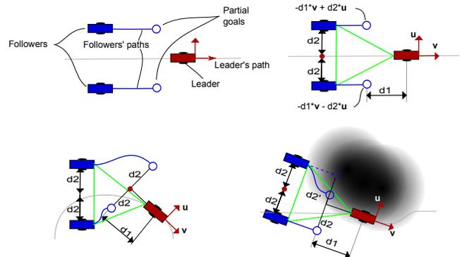
Fig. 4: Top left - Main components of the robot formation algorithm. Top right - Reference geometric definition of a simple, triangle-shaped robot formation. bottom left - Behaviour of the partial goals depending on the leader's pose. Bottom right - Behaviour of the partial goals depending on the obstacles of the environment.
