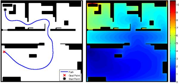
Fig. 3: Example of a path obtained with the FM<sup>2</sup>. The left side shows the resulting path of the algorithm in the initial map. In the right side there is the time of arrival map.
