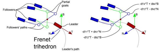
Fig. 6: Schema of the definition of the geometry in 3D based on the Frenet trihedron.
