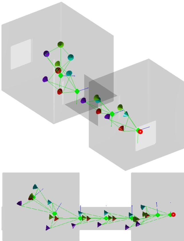
Fig. 9: Example of a motion sequence in a narrow corridor, leveraging the priorities introduced in the algorithm. Top: 3D view. Bottom: top-view which allows to see how the robots change their relative position in the direction of the motion.
