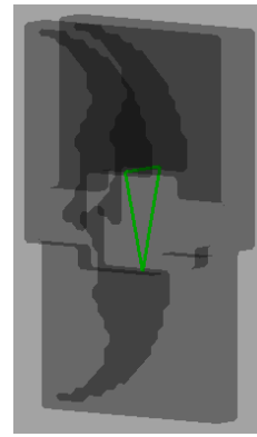
Fig. 8: Environment matrix with the addition of the workspaces of the fingers.
