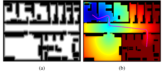
Fig. 5: a) Saturated slowness potential F(x) . b) Second wave expansion D(x) and the path obtained. Note that the level lines and the path are not equal than in figure 4.
