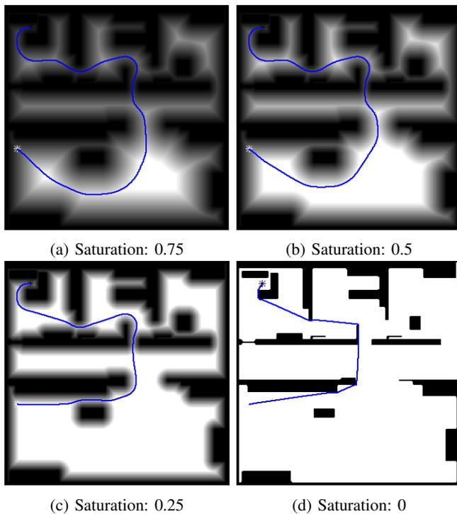
Fig. 3: FM<sup>2</sup> saturated variation: modification of the path depending on the saturation value.
