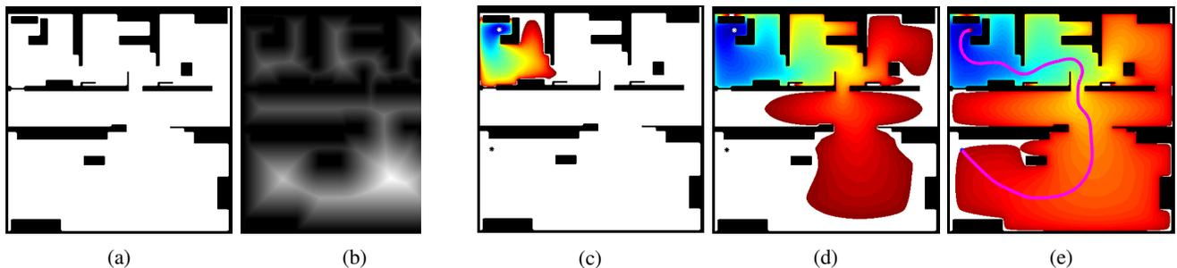
Fig. 2: Steps of the FM<sup>2</sup> algorithm. a) Initial binary map. b) Velocities map generated with FMM. c),d) Wave propagation from the goal point. e) Final path shown over the time-of-arrival map.
