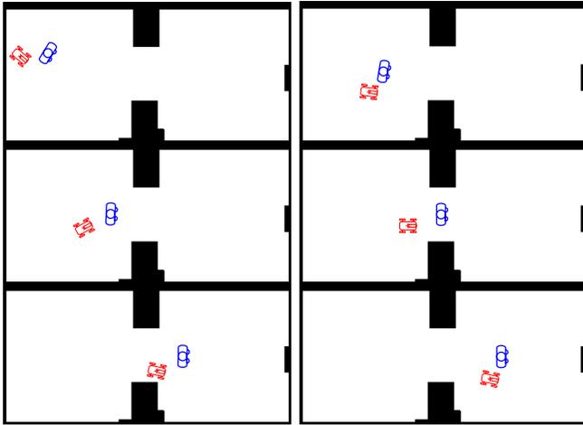
Fig. 7: From top-left to bottom-right: sequence of a robot following a human with the FM<sup>2</sup>-based robot formation motion planning algorithm.
